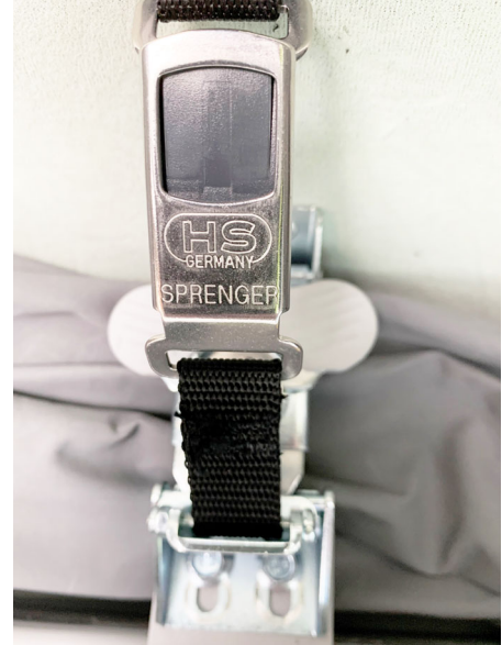
Ensure that the turn knobs are folded back up and the retention clamps are secured before travel. -Typical View
