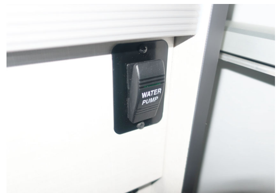
Water Pump Switch in the rear of the galley. -Typical View
