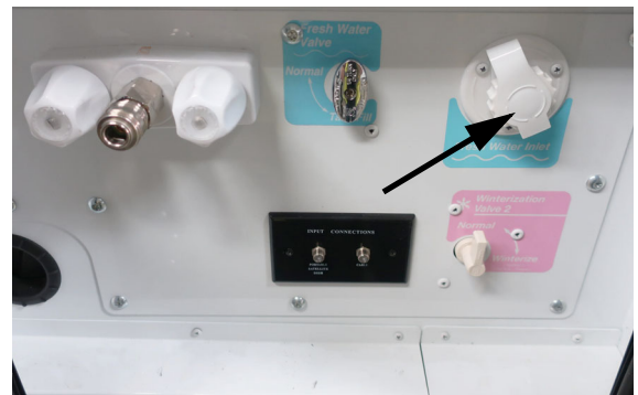
City Water Inlet (Located behind the drivers side Water Service Center door) -Typical View
