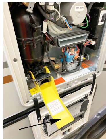
Water heater Easy Drain Lever in lowered position. -Typical View
