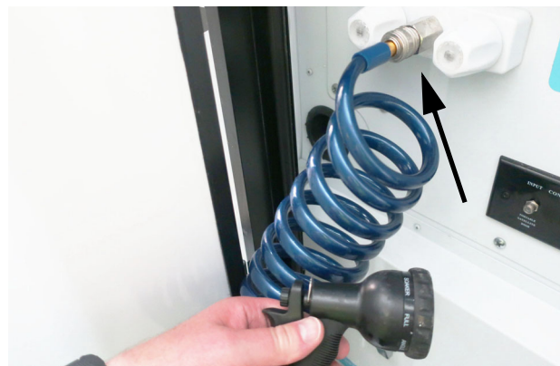
Exterior Shower/Wash Station (located in the drivers side Water Service Center. -Typical View)
